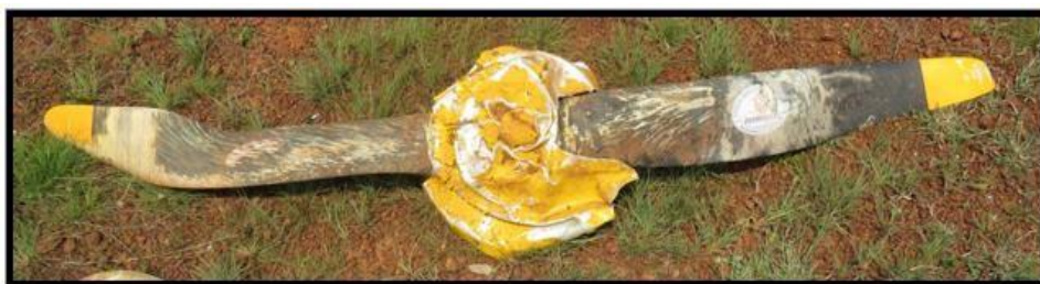
Fig 5: Rubbing marks on Propeller
