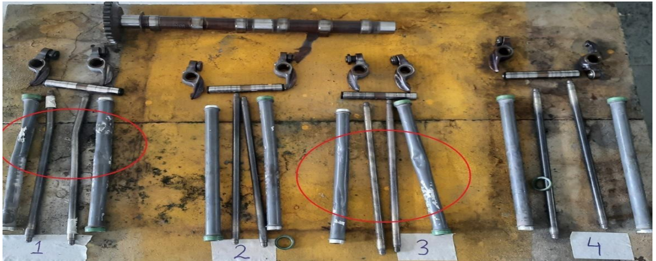
Figure: 13 Push rod, shroud, rocker arm, rocker pin & camshaft
