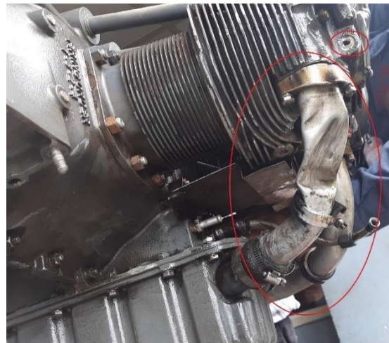
Figure: 4 Induction tube (Cylinder 2 & 4) and sheared rocker box oil elbow.
