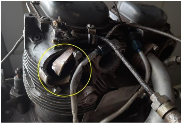
Figure: 8 Induction tube (Cylinder no. 1) and broken mounting flange with missing tube
